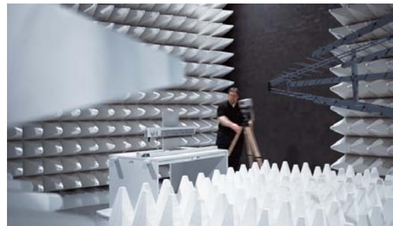
Fig. 1: Testing the electromagnetic compatibility of valves in Festo's EMC laboratory
