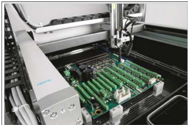
Fig. 4: The compact planar surface gantry EXCM guides the test probe accurately to the test points on electronic modules.
